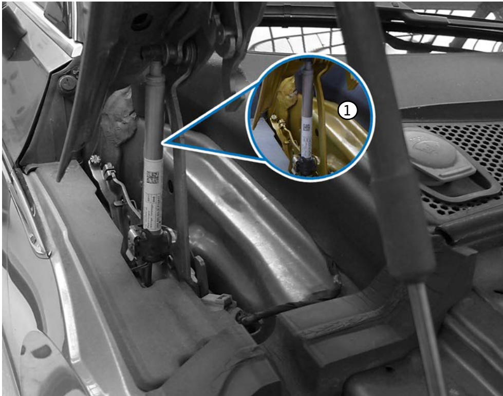
Example of a re-active hood with pyrotechnic actuator.
