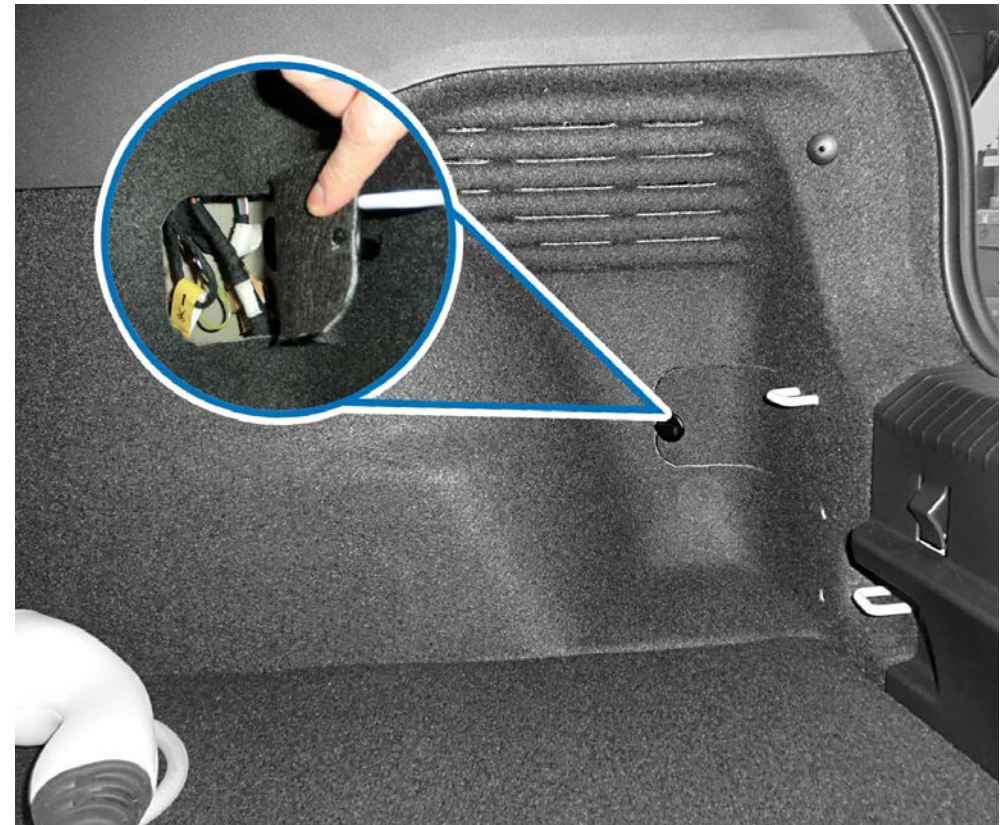
Variant 1: Disconnect high voltage device in luggage compartment (example ID.3) behind the side panel trim up to the end of 2020. The yellow flag indicates the cut-off point.
