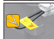
Pull out or cut the high-voltage cut-off switch (A) to deactivate high voltage.
