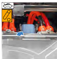
Disconnect from the charging station (emergency release)
