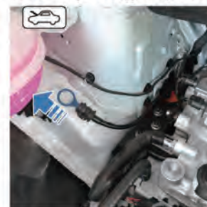
Disconnecting from the charging station (emergency release)
