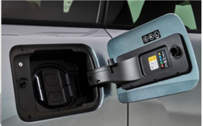
High-voltage charging socket at the right rear side panel
