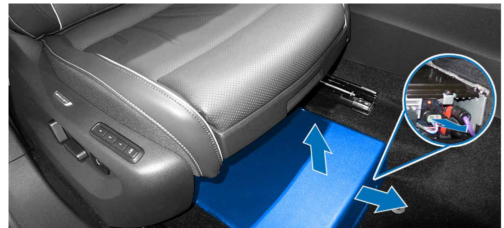
Disconnecting the 48-volt vehicle electrical system in a Tiguan from 2023 onwards.
