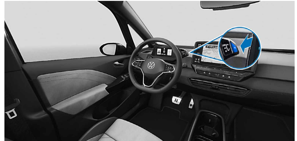
Vehicle of ID. family: operate the electronic parking brake on the right-hand steering column switch.
