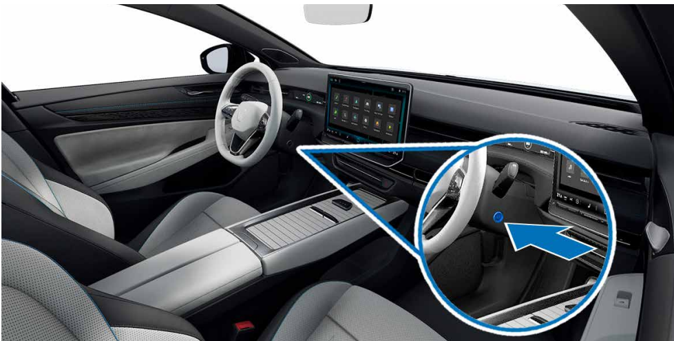
Vehicle with START-ENGINE-STOP button on the steering column.
